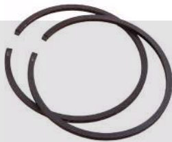
Spheroidal cast iron piston rings, typically used only in racing engines, for improved compression.
