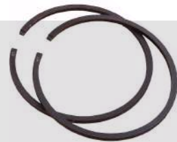
Spheroidal cast iron piston rings usually used only in competition engines, which ensure better compression.
